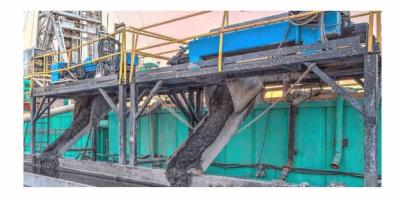
**Process/Solution:** We would tie into the 3-inch line coming off your 6-inch line that feeds your filter presses with thickener tank underflow. Thickener tank underflow would move down the 3-inch into our dual centrifuge set up. This will ensure that we have ZERO impact on your operation
