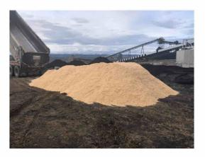
An end dump (20 m3) of sawdust was purchased to demonstrate it's effectiveness in absorption of moisture and its usefulness in creating an end product that is cohesive enough to be driven on top of and moved with a D7 Cat dozer, all while reducing the need for or eliminating the use of additional haul trucks and large excavators on the refuse pile.
